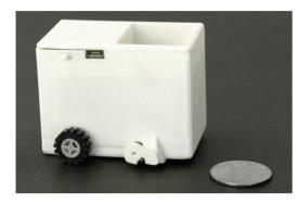
Meet Sustainabot: a small robot printer that deposits everyday materials - foodstuffs, powders and so on - on flat surfaces to create patterns and shapes directly from a mobile device.
