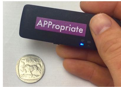
**Figure 4.** The APPropriate hardware, with a 5 Rand coin for scale. A switch on the side of the device (next to the user’s fingertip in the photo) toggles its inbuilt WiFi on and off. The blue light in the image flashes on startup, then goes constant once ready to sync.
