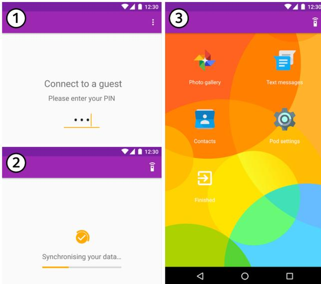
**Figure 3.** The APPropriate app interface on a borrowed phone. Picking up any APPropriate-enabled Android device prompts for a PIN (image 1). Entering the correct PIN authenticates with the user’s APPropriate module and synchronises their content (2), presenting as closely as possible the same experience (photos, SMS messages, contacts and wallpaper) that the user is familiar with on their own smartphone (3).
